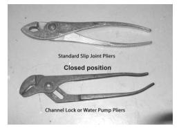
screws have right hand threads. This means they go clockwise to tighten and counter clockwise to loosen, or as known in the trade, "righty tighty and lefty loosey". Be sure to hold and turn the water pump pliers and or the adjustable wrench the right way or they will slip. The water pump pliers should be in a position in the adjustable grooves that allows you a good grip
